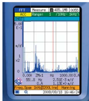
Spectrum display (3 200 lines)
